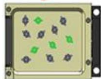
Vision system (SmartSight) detects which parts are correctly oriented
